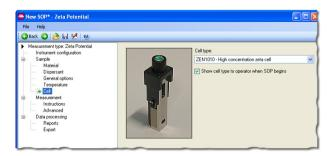
When using the High concentration cell select the cell in the relevent **Cell** SOP window.
